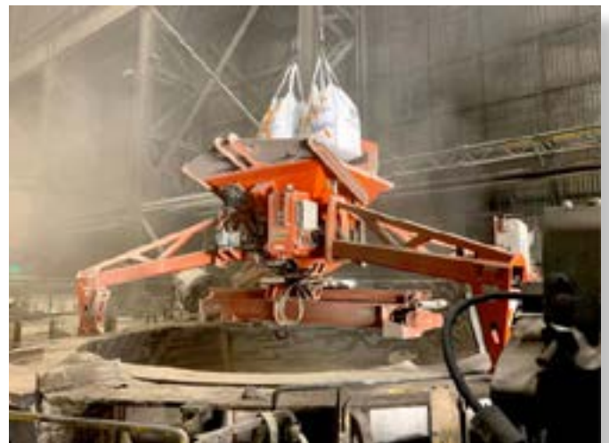
Fletcher Model SS-1 Bottom Hearth Material Spreader
