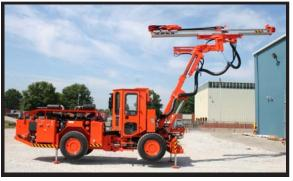
J. H. Fletcher & Co. has long been known for designing machines to meet specific mining applications or needs of the customers. When a customer approached us about needing a narrow machine to drill the face in a copper mine, Fletcher met the need by designing the J-151 DE Narrow Vein Drill Jumbo.
